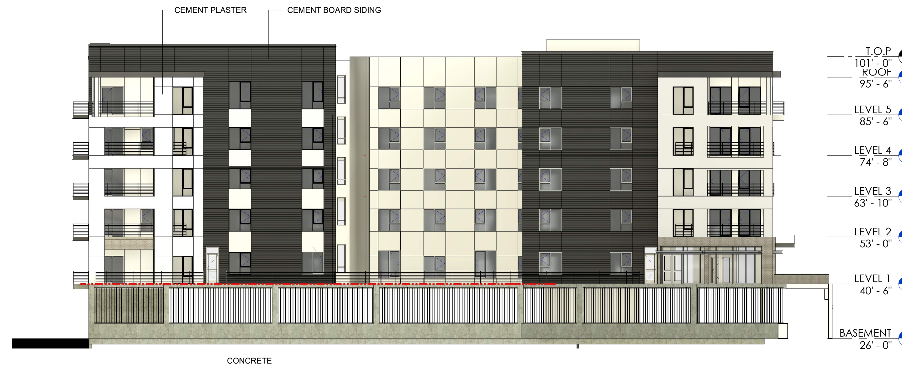
SOUTH ELEVATION (SERVICE ACCESS)
